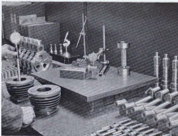
*Inspection. — Here the product has to undergo the severe scrutiny of the fixed tolerance.*
